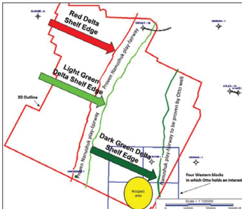
The prospect, identified on modern 3D seismic data obtained through the Alaska Department of Natural Resources, Division of Oil and Gas, is illustrated above in the context of the four graticular leases that comprise the Western Blocks in which Otto holds an interest.
